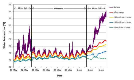
**Figure 2.** Data from the PAX Water Mixer in a 4MG tank shows that the water temperatures became uniform within 0.5  $^{\circ}$ F. When the mixer was turned off, the tank quickly became thermally stratified.
